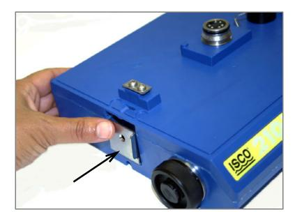
Latches will "click" when they are fully locked or unlocked.
