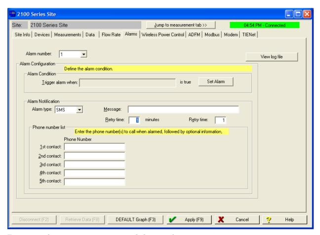
Figure 2-16 Setting up text messaging and alarm conditions
