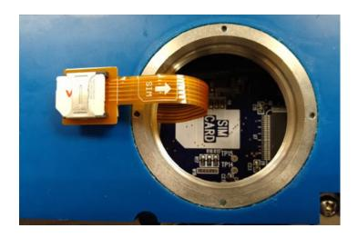
Figure 3-4 Inserting the SIM card
