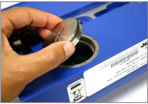
Figure 3-2 Accessing the SIM card on the bottom of the module
