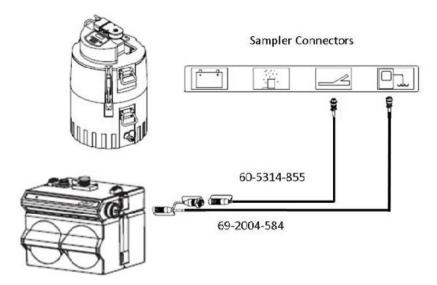
Figure 2-22 Cable connections for sampler Pass-Through Mode
