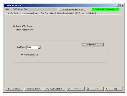
Figure 2-27 ADFM tab for Pulse Doppler devices
