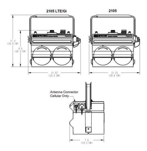
Figure 1-6 Specification drawing: 2105 mounted on 2191 battery module
