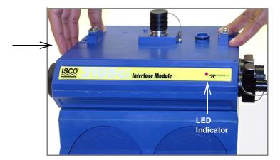
Figure 2-7 Aligning the modules
