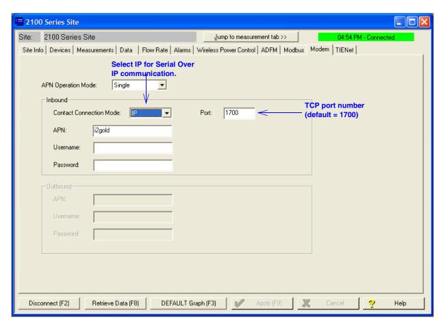
Figure 2-12 Modem screen - configuring the cellular modem
