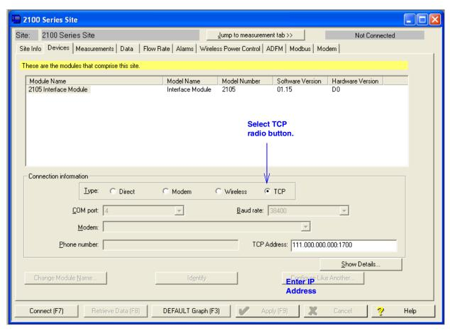
Figure 2-13 Devices screen - configuring for Serial-Over-IP communication
