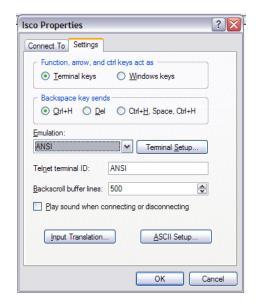
Figure 2-25 HyperTerminal Settings tab
