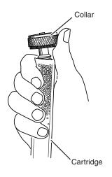
The desiccant is contained in a cartridge located on the side of the 2105. To remove the cartridge, unscrew the collar and slide the cartridge out of the 2105. The clear tube reveals the silica gel desiccant inside.
