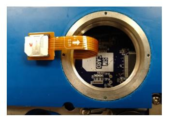
Figure 4-4 Inserting the SIM card
