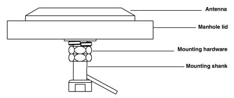
Figure 4-8 Manhole lid-mount antenna
