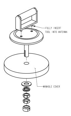
Figure 4-9 Manhole lid-mount antenna: Installation
