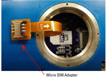
Figure 3-3 SIM card extender and Micro SIM adapter
