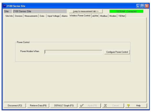
Figure 2-14 Wireless power control window with no program scheduled
