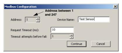
Figure 2-29 Modbus configuration window
