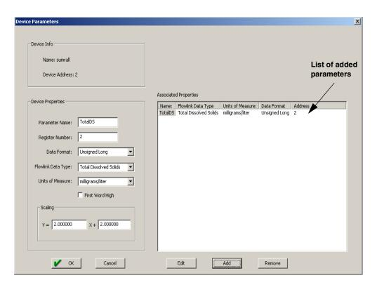
Figure 2-30 Device parameters (measured data)
