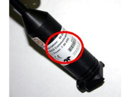
Figure 2-2 Identifying the voltage specification on the DB9 cable
