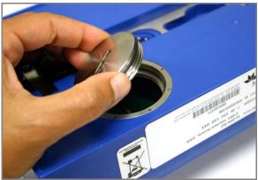
Figure 4-2 Accessing the SIM card on the bottom of the module
